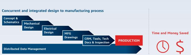
At the center of this solution is a shared 3D CAD model, enabling design or manufacturing changes to be effectively managed and allowed to propagate automatically to all related drawings, downstream manufacturing systems and technical documentation that are affected by the change.
