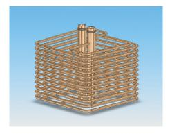
With SolidWorks software, Fernstrum can use design tables to develop different configurations from a standardized heat exchanger design.
