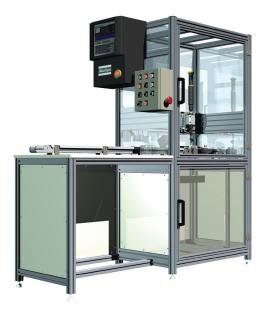
ACPA manufactures special purpose machinery, such as a sensor for detecting side crashes for the automotive industry. Shown here is the ACPA Semi-Automatic Screwing Machine.
