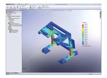
Using the integrated SolidWorks Simulation structural analysis software, engineers can validate machine performance and ensure that their products will withstand the duty cycle required by their customers.
