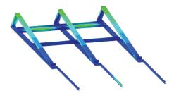
With SolidWorks simulation tools, SunEdison studied the effects of structural and wind loads, validating system performance quickly and cost-effectively.
