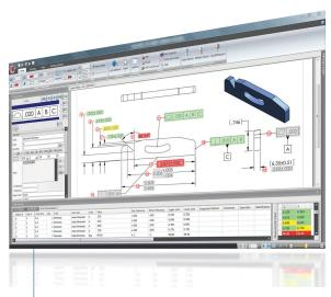
Characteristics are automatically highlighted in green, red, or yellow to instantly show which are in tolerance, out of tolerance, or marginally within tolerance.
